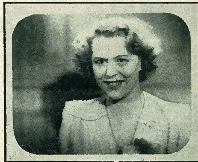
Fig. 1 "Ringing" in Line Time Base, causing vertical dark bars on left of picture.
