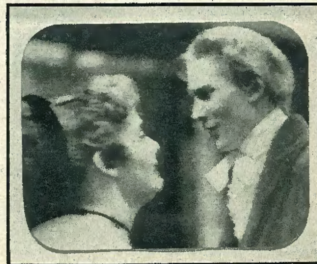
Fig. 2. Non-linearity of Line Time Base, causing extension of left-hand side of picture.
